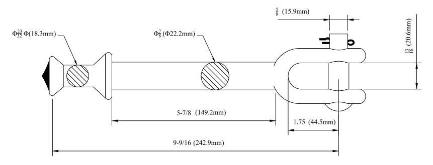
HOT LINE BALL CLEVISES ARE USED TO ATTACH BALL AND SOCKET INSULATORS TO OTHER ASSOCIATED HARDWARE WITHIN AN INSULATOR STRING. SHOULDERS ARE PROVIDED TO ACCOMMODATE HOT LINE TOOLS.
