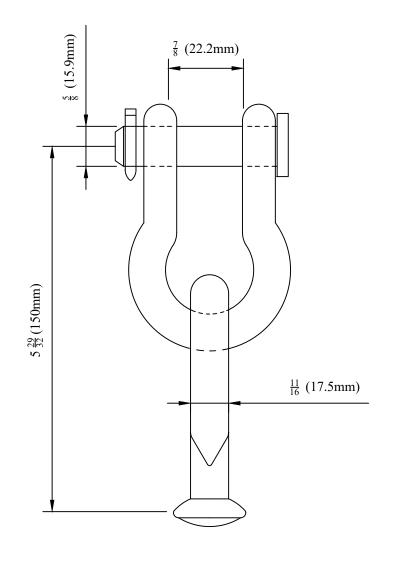
BALL OVAL-EYE ANCHOR SHACKLE COMBINATIONS ARE POPULAR COMBINATIONS WHICH ARE SOLD AS ASSEMBLIES TO SAVE FIELD ASSEMBLY TIME. CONTACT FACTORY FOR OTHER PRE-ASSEMBLED COMBINATIONS.
