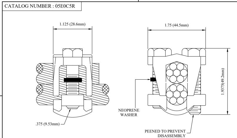
FOR COPPER TO COPPER CONDUCTOR CONNECTIONS.
