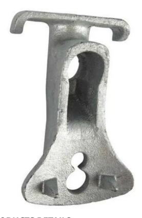
Cast Ductile Iron Guy-Hook Attachment For Deadending Guy Wire, 33,500 lbs. Strength, 1" Bolt Size with 9/16" & 13/16" LOWER HOLES
